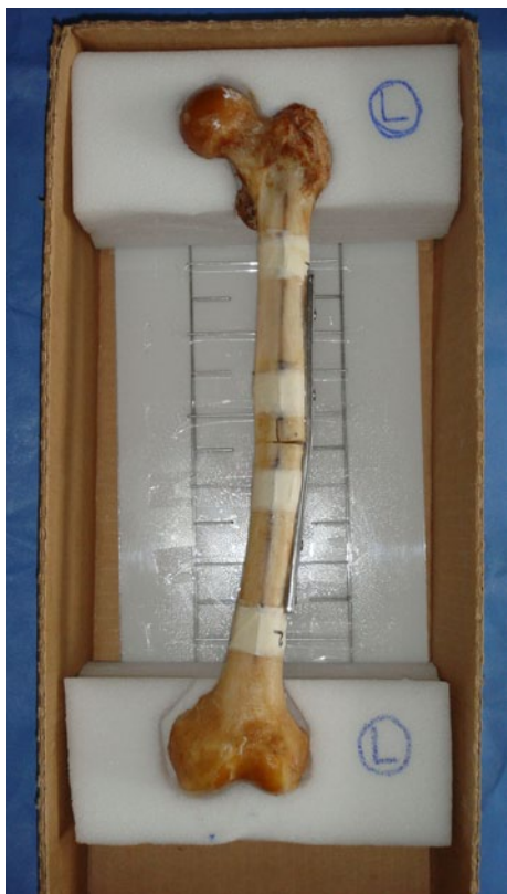
Fig. 2 The angulated femur fixed with broad DCP was placed in the box over the alignment grid
